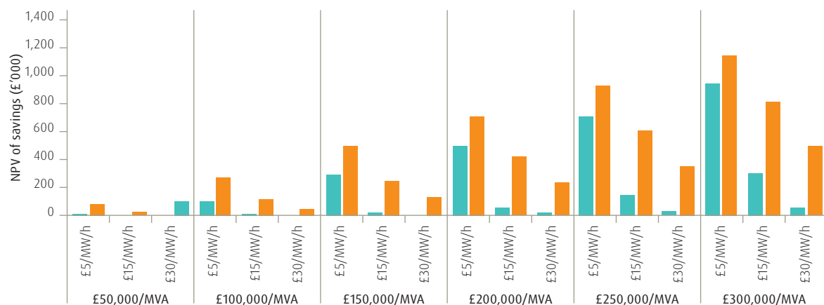
Figure 1: Cumulative savings at Clapham Park Road NPV (£'000) for different DSR availability prices and network reinforcement costs
